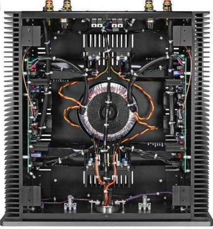
Despite its relatively low power, the Sugden uses a substantial power supply to achieve its 30+ Watts of Class A operation. Large heatsinks are need to dissipate the heat produced by Class A. whilst keeping temperature down. The amplifier is more efficient than standard Class A, being a circuit pioneered and developed by Sugden.
